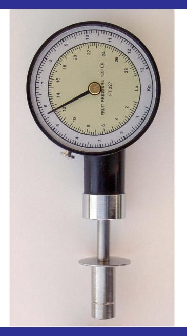
This small and very manageable tool is perfectly fit to detect proper picking maturity and control fruit softening during cold storage. Fruit firmness is the universally accepted measure of ripeness and the FT Fruit-Tester is the world wide recognized tester.
